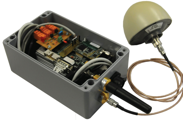
Fig. 3. Prototype implementation housed in waterproof enclosure (60x100x160mm) with power connector, and external radio transceiver and GPS (Trimble Bullet III) antennas
