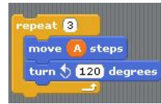
Figure 6: The program from Subfigure 2b, with the length of each side replaced by the variable A .
