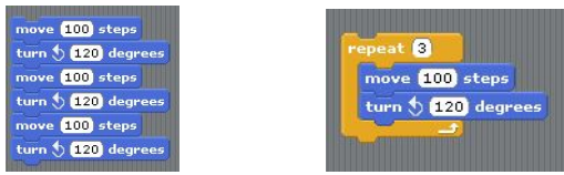
(a) Blocks to create a regular triangle, step by step. (b) The same construction, but now with a loop.
