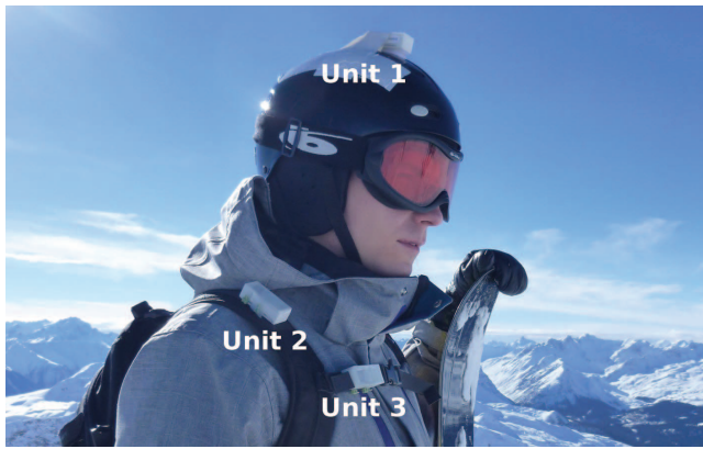
Figure 9. Positioning of the three wearable sensor units during the field experiments: Unit 1 is attached on the helmet, Unit 2 is attached on the shoulder, and Unit 3 is attached near the chest. The sensor units are enclosed within a plastic housing to protect them from snow.
