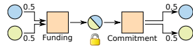
Fig. 1. Construction of a micropayment channel. The boxes are transactions or a number of transactions and the circles are outputs. The colors in the circles describe whose signatures are needed to spend those outputs. To spend an output belonging to multiple parties, all of those parties must sign. The lock indicates unspent transaction outputs on the blockchain while the channel is open.
